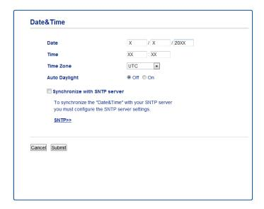
• Choose the **Synchronize with SNTP server** check box. You also need to verify your time zone settings correctly. Choose the time difference between your location and UTC from the **Time Zone** pull-down list. For example, the time zone for Eastern Time in the USA and Canada is UTC-05:00.
